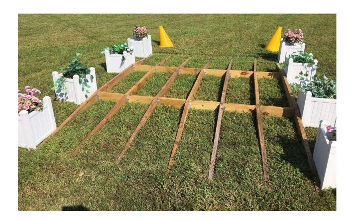
4. I like to keep mine portable, so I pre-drilled holes for 3" deck screws to be set in at an angle, to hold the 14" spacers in place to the long plank, and when I'm done, I back the 3" screws out and can store the whole thing away. I leave the joist hangers in place, so never need to measure again. Blue line shows how long screw is set in at angle to anchor cross piece.
